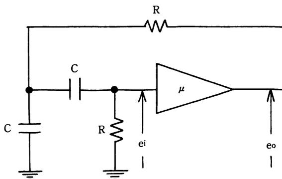
Fig.1 RC oscillator
