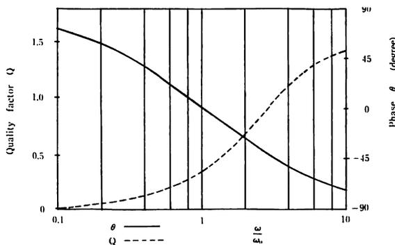
Fig.4 Quality factor and phase characteristics of the circuit of Fig.1
